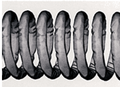
PHOTO OF NOTCHING PHENOMENON
